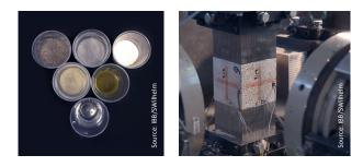
The pressure housings are manufactured using UHPC (Ultra High Performance Concrete) – a material that is characterized by its high compressive strength of over 160 MPa, which currently allows the use of the pressure housings at depths of up to 6,000 meters. The concrete has an extremely dense structure, making the pressure housing watertight even in great depths.
